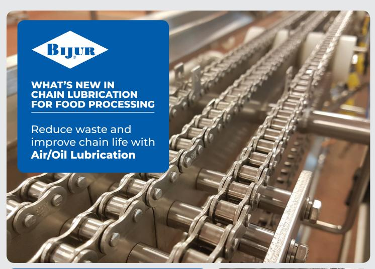
Air/Oil systems with their precise delivery are 90% efficient compared to mist systems 60% efficiency. Reduce waste with Air/Oil.
